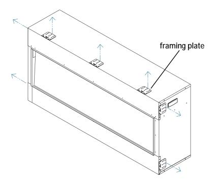
3. Re-attach the framing plates as shown in the picture.
