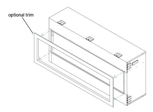
2. Remove the framing plates from the unit.
