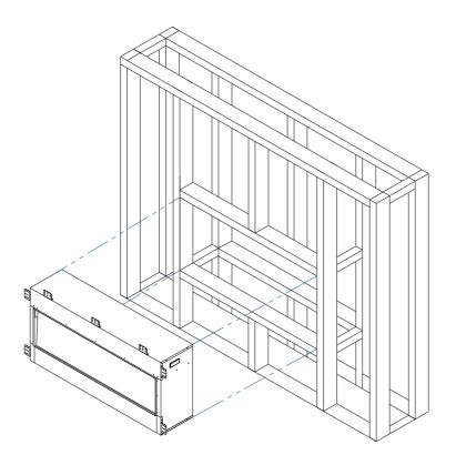
6. Drive the mounting screws into the framing plates on the unit and the wall studs.
