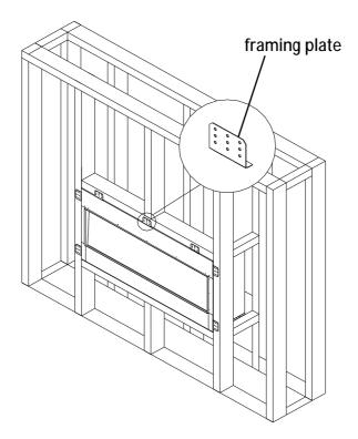
7. After checking that the fireplace operates properly, cover the glass panel with protective plastic bag and install plywood or drywall.
