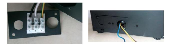
3. Return the cover plate to the left side and screw the two screws back in to fasten the plate.
