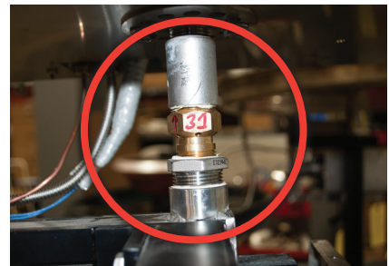
Figure 9.1 – Locating orifice for cleaning
