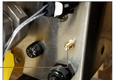
Figure 6.9 – Attach antenna cable
