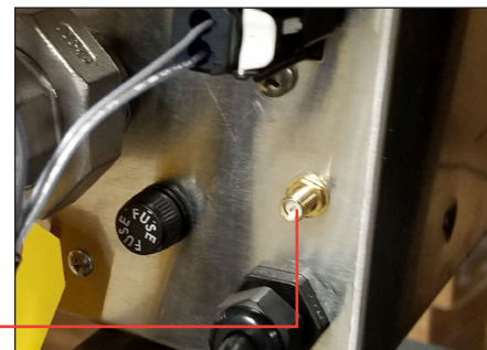
Figure 6.5 – Attach antenna cable
