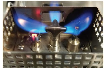
Figure 9.2 – Pilot flame coverage of thermocouple.
