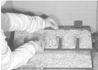
Figure 8c- Placing rock wool
