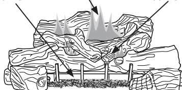
Figure 46 - Incorrect Burner Flame Pattern
